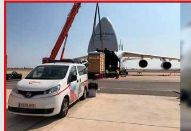
CARGA Y TRINCAJE EN ANTONOV AN-124
